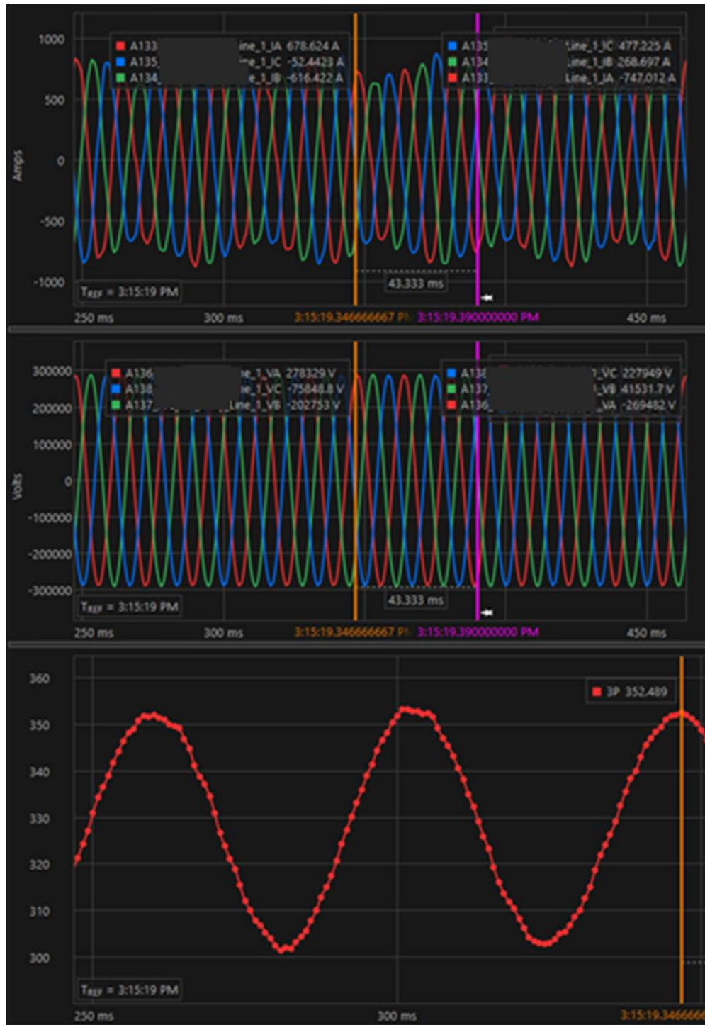
Figure 2. Large load oscillation event at ERCOT observed from 20 samples/cycle DFR measurements. The red trace in the bottom plot is three-phase power and reveals the 50 MW oscillation. Source: ERCOT (Gravois 2025).
